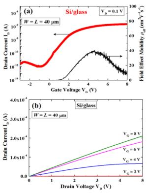
**Figure 3.** (a) Transfer and (b) output characteristics of a fabricated poly-Si TFT for <u>Si/glass</u> structure with W = $L = 40 \ \mu m$
