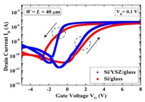
Figure 5. Hysteresis phenomenon occurring in the transfer characteristics of fabricated poly-Si TFTs with  $W = L = 40 \ \mu m$  at  $V_D = 0.1 \ V$  for the two structures of the Si/glass and Si/YSZ/glass
