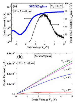
**Figure 4.** (a) Transfer and (b) output characteristics of a fabricated poly-Si TFT for <u>Si/YSZ/glass</u> structure with  $W = L = 40 \ \mu m$
