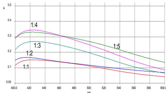
**Fig. 3.** UV spectrum shows effect of the mixing ratio of extract volume/ 1 mM  $\text{AgNO}_3$  solution volume in the silver nanoparticles synthesis
