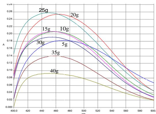
**Fig. 2.** UV spectrum shows effect of the ratio of lemongrass leaves weight/distilled water volume in the silver nanoparticles synthesis.
