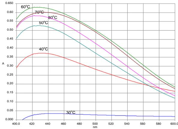
**Fig. 5.** UV spectrum shows effect of temperature in the silver nanoparticles synthesis
