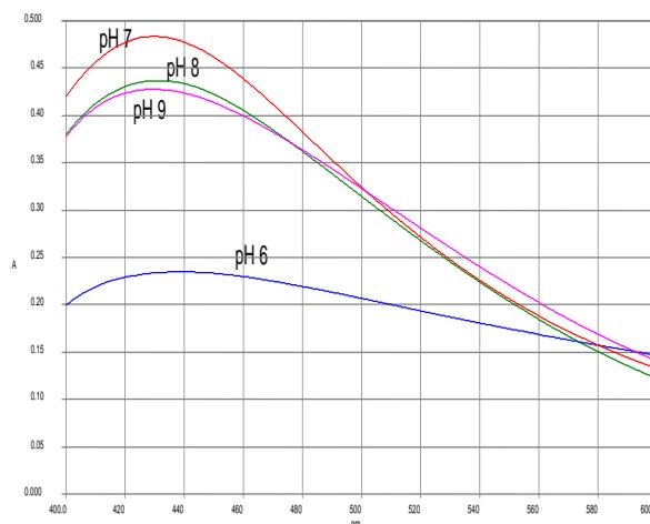
**Fig. 4.** UV spectrum shows effect of pH on the formation of silver nanoparticles
